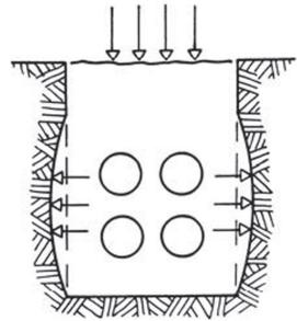
Figure 4.1 Trench Conditions in Soft and Unstable Soils
