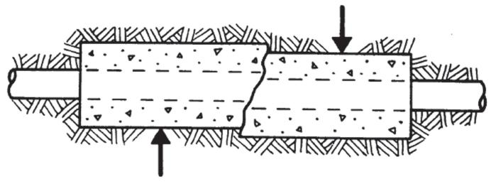
Figure 1.3 Conduit bank damaged through shear forces on concrete
