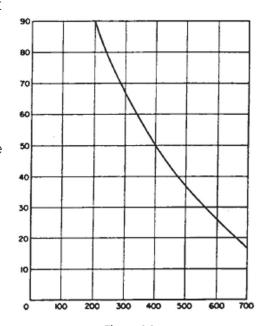
Figure 2.3 Approximate Relationship Between Angular Deflection and Length of Run
