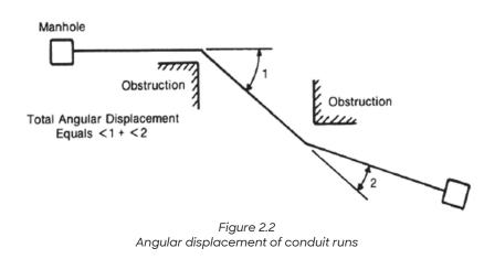
When laying out the proposed conduit run, one should strive to keep the route as straight as possible. Where direction changes are indicated due to obstructions in the route, the angular displacement should be maintained as small as possible. The total angular displacement of the conduit run is determined by adding up the angles of each direction change to find the sum total, as can be seen in Figure
