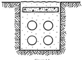
Figure 1.4 Direct burial with cover slabs
