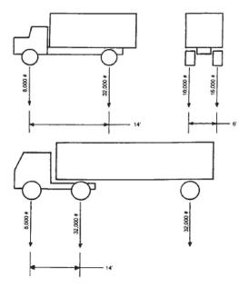
Figure A-1 AXLE WEIGHT DISTRIBUTION FOR H-20 LOADING
