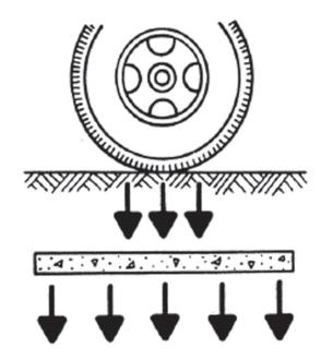
Figure 1.5 Load distribution with cover slabs
