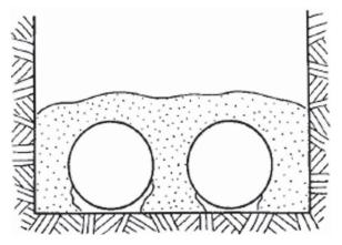
Figure 4.2 Lack of Fill Material Under Conduit Haunches Due to Improper Installation Procedures
