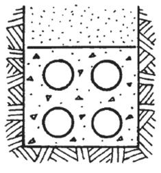
Figure 1.1 Concrete Encased Conduit Bank
