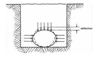
Figure 3.3 Loading on Buried Conduit
