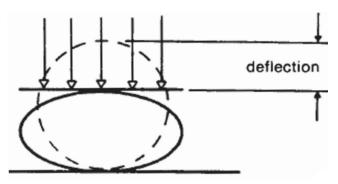
Figure 3.2 Parallel Plate Loading Test in Free Air
