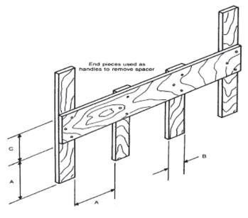
Figure 4.5 Wooden Comb Type Spacer
