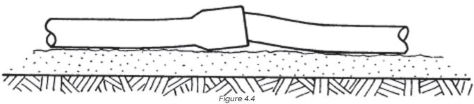
Improper conduit alignment due to lack of excavation at joint
