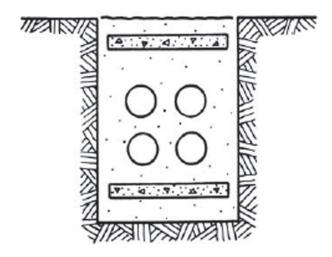
Figure 1.6 Conduit bank with upper & lower concrete slabs
